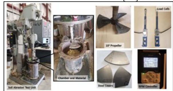
Figure 1 Components: Soil Abrasion Test Machine
